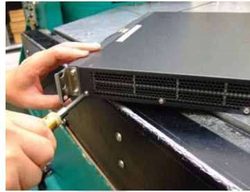
Figure 4.89 Example of checking result of Vibration test
