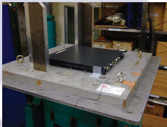
Figure 4.88 Example of assigned work of Vibration test
