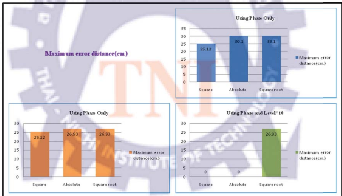
Figure a-16 The maximum error distance of phase, power level and summation of phase and power level(x10) information with equations 3.1, 3.2 and 3.3
