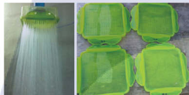
Fig. 8 The super lock box modified to be spray nozzle of the cooling tower (with 2.5, 3.0, 3.5 mm holes)
