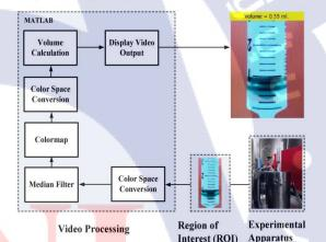
Fig. 3. Diagram of overall operation procedures through video processing technique, showing the region of interest (ROI), video processing in MATLAB and output capture.
