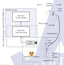
Fig.2. Diagram of the proposed semi-automated radiopharmaceutical dispenser with real-time video processing.
