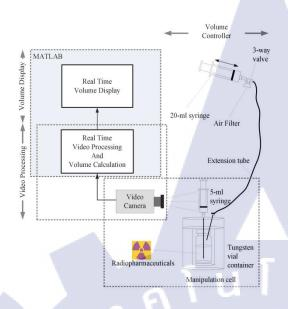
Fig. 2. Diagram of the proposed the realization of real-time video processing for volume mesurement in radiopharmaceutical dispenser.
