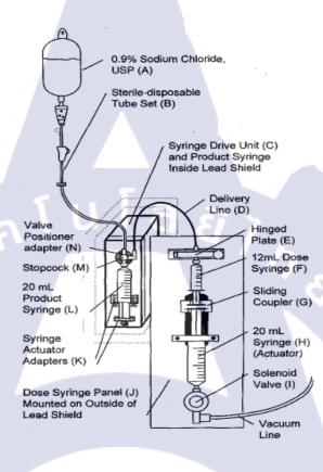
Figure 2.13 Layout of assembled dispensing unit.
