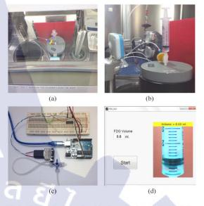
Fig. 5. Photographs of experimental set-up and demonstrations; (a) the original beveling view of a manipulation cell that is visible for the operator, (b) the proposed video camera with close distance, (c) the prototype of the proposed system, (d) the GUI of the proposed system.
