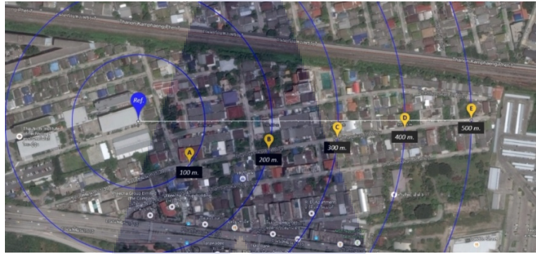
Figure 4.4 Test for signal strength coverage area at C-Building of Thai-Nichi Institute of Technology
