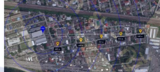
Fig. 7. Test for signal strength coverage area at C-Building of Thai-Nichi Institute of Technology.
