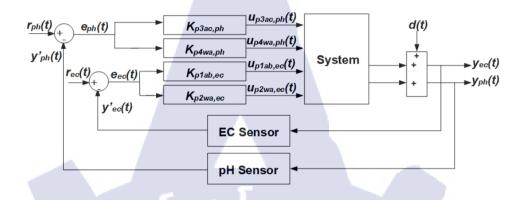
Figure 3.24 P control for EC and pH control block diagram
