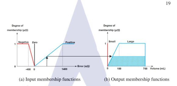
Figure 3.6 Defuzzification in modified fuzzy logic control.
