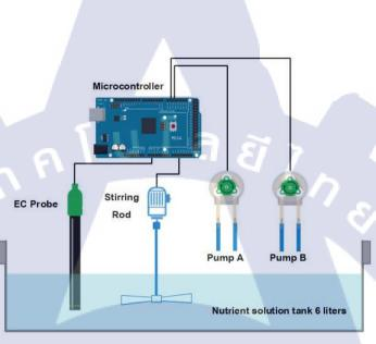
Figure 3.8 EC control equipment
