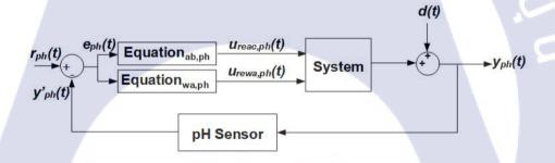
Figure 3.16 Linear regression block diagram for pH control
