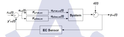
Figure 3.10 P control block diagram for EC control
