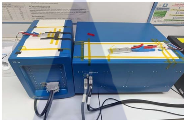
Figure 3.2 Biologic VSP-3e Potentiostat/Galvanostat connected to VMP3B current booster
